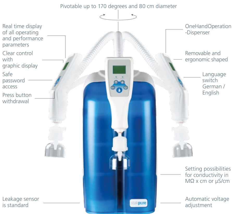
Autonomous specialist with integrated pre-treatment and ultrapure water cartridge. Simple cartridge change in seconds.
